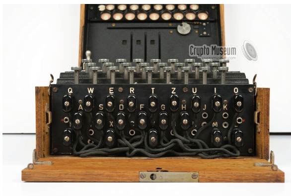
FIGURE 10.4: Enigma – plugboard (courtesy of www.cryptomuseum.com )
