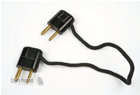
FIGURE 10.5: Enigma – plugboard cable (courtesy of www.cryptomuseum.com )
