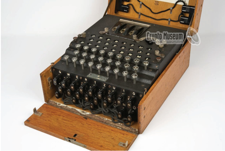
FIGURE 10.1: Enigma – Model I (courtesy of www.cryptomuseum.com )
