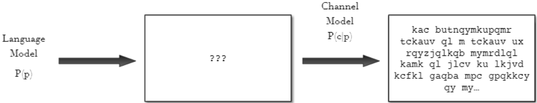
(b) In a ciphertext-only attack, we only have the ciphertext, and we want to find the plaintext. We model the plaintext generation process by an English language model P(p) that assigns a probability to each English string p , and we model the encipherment process by a channel model P(c|p) that assigns a probability for each character substitution
